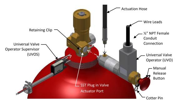
**Figure 3 UVO Kit Component Installation**
