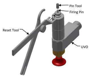
**Figure 5 Reset Tool Alignment**
